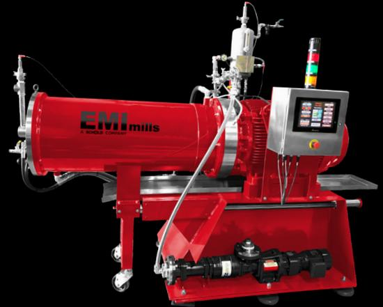
150L Mill with PLC Controls
